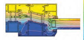
example isotherm distribution for the combination of a frame and a window sash in the IP OUT i+ system (IP O10 + IP 521)
